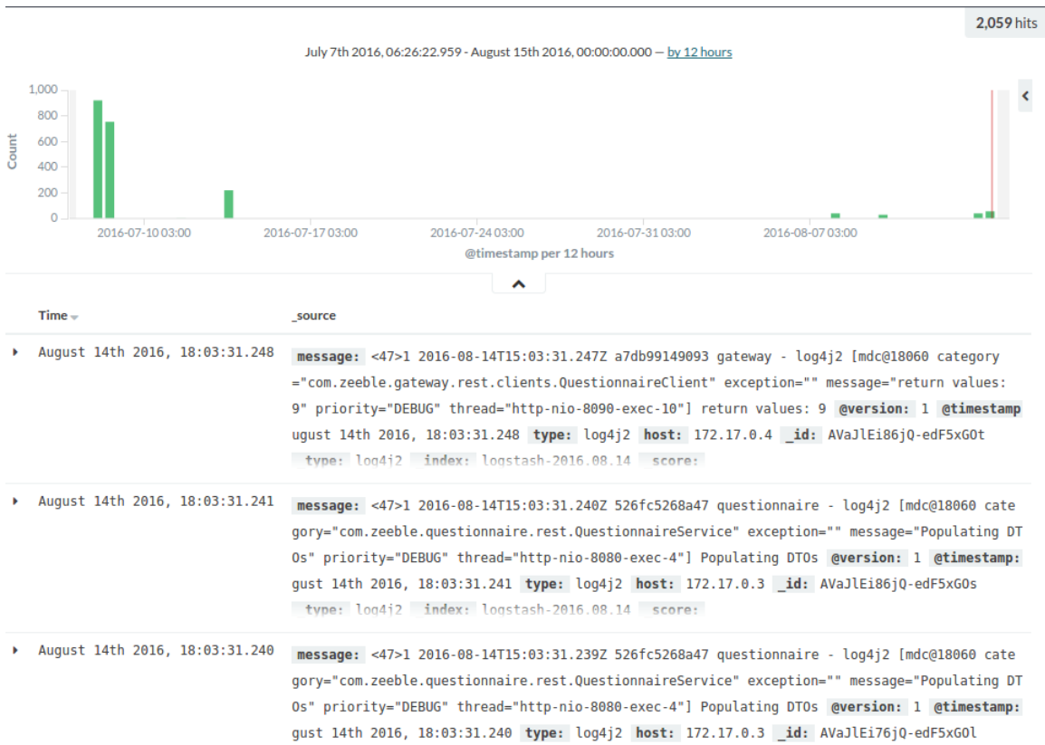
Figure 7: All log events visible in the main screen with count graph over time
