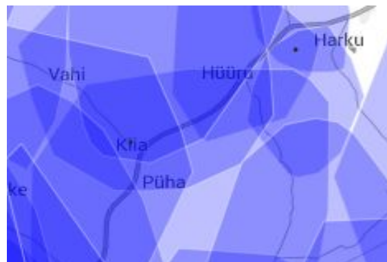
Cell coverage area calculated by specialized planning software used by operators
