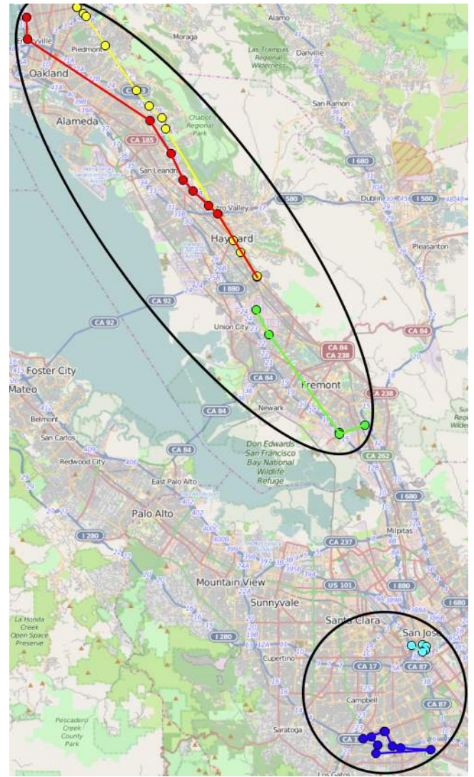
Figure 3: Clustered clusters of cell points with combination of DBSCAN and hierarchical algorithms. Ellipses represent main clusters. Points with same color are in one sub-cluster.
